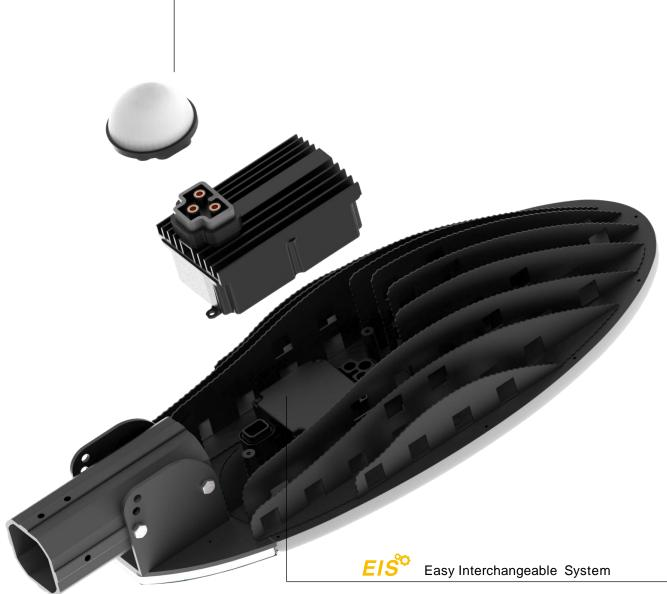
Structuring the heat sink into compartments with multi-directional heat dissipation fins will increase the total surface areas; greatly enhance efficency to dissipate heat from the light, the air channels are designed to let air flow through the fins and take away the heat as well as to drain away dust and water from accumulating on the fixture effectively.
